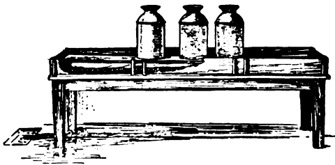
FIG. 82. — Draining rack with milk cans full of water used for pressure.
